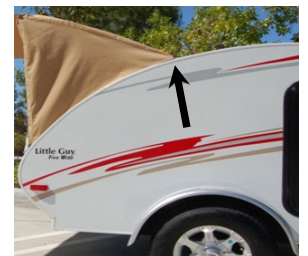
Front edge of Hatch Cover/Awning
